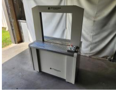
Plastic Strapping Machine 28" Tall x 24" Wide Strapping Area
